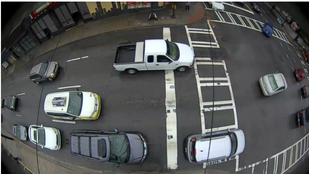
Sensor detection: vehicles parked in crosswalks
